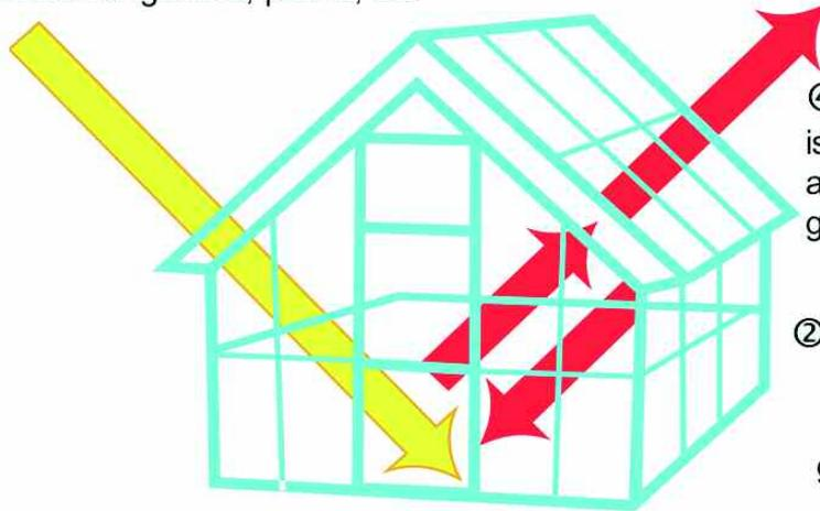
④...but some IR energy is reflected by the glass and trapped inside the greenhouse.
